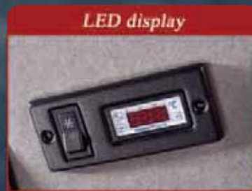
LED display to control cargo bay temperature
